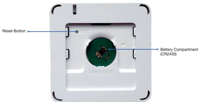
[Image 4] Wall switch Hardware Version 2 (With Reset Button)
