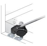
Recommended fixing 2 pan head wood screw  $\emptyset$  4 x 15 mm
