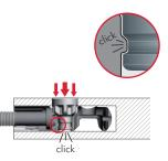
Press strongly with PZ2 cross screwdriver to slot the pinion screw in.
