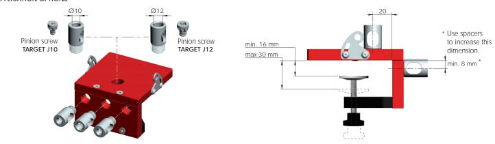
DRILLING SPACERS FOR OTHER PANEL THICKNESSES
