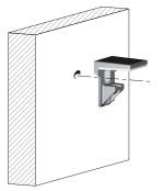
Recommended fixing countersunk screw type - head  $\emptyset$  5 mm max.
