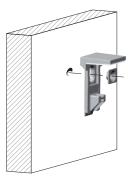
Recommended fixing countersunk screw type - head  $\varnothing$  5 mm max.
